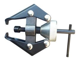
Adjustable tool for quick and easy removal of wiper arms.
